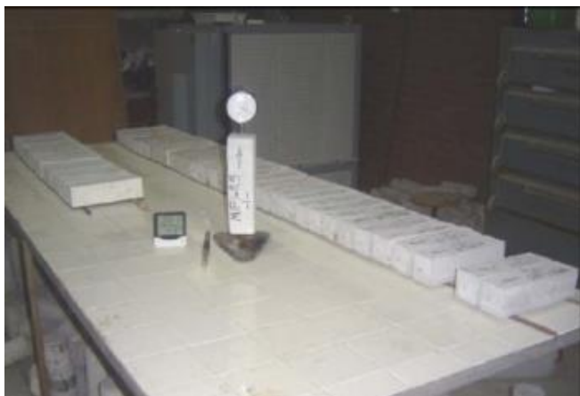
Obr. 7: Drying shrinkage test
